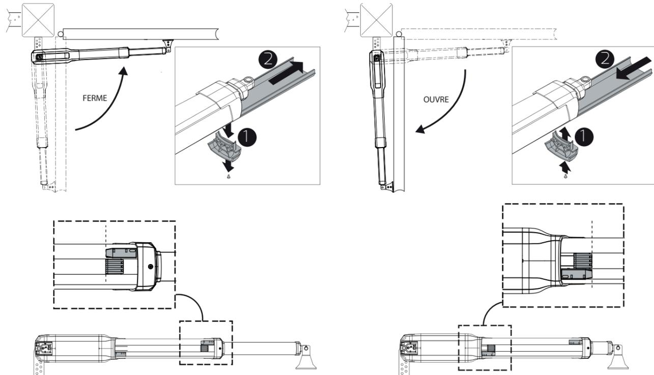
Adjust the limit switches and the stops according to the diagrams, open/closed position.
