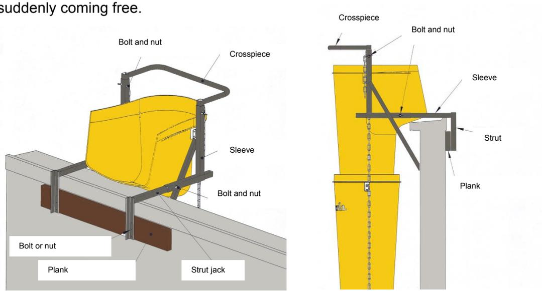
The chute sections can now be mounted to the window fixing frame.
