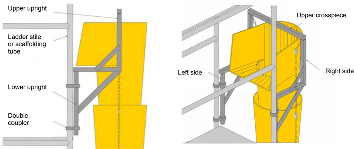
The chute sections can now be mounted to the scaffolding fixing frame.
