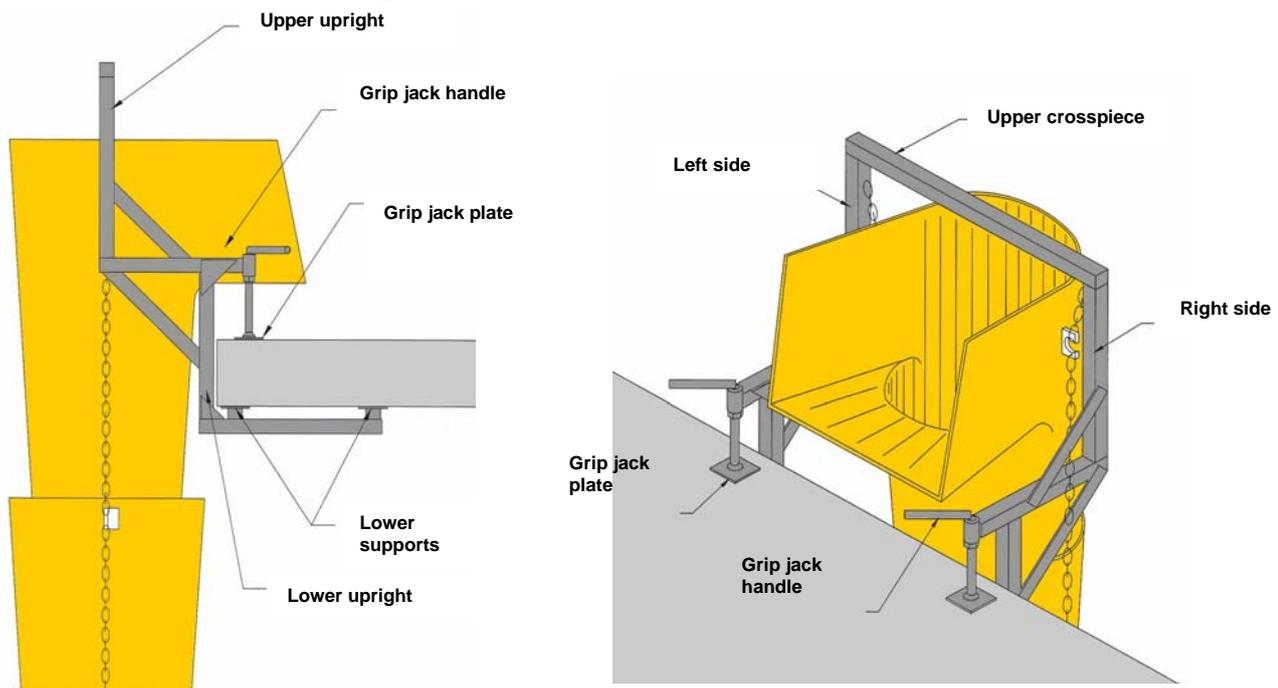
The chute sections can now be mounted to the platform fixing frame.
