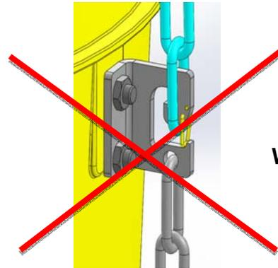
Anchor the rubbish chute to the building using a rope or a chain every 10m (30ft).
